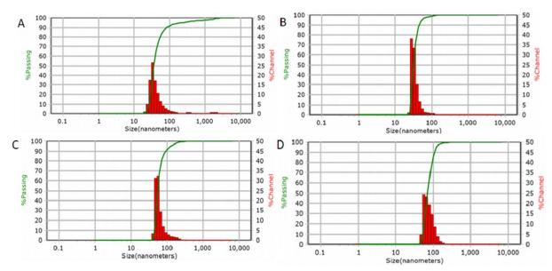
**Figure 1.** measuring the diameters of nanoemulsion particles in different treatments. A: Nanomulsion containing 1% extracts, B: Nanomulsion containing 2% extracts, C: Nanomulsion containing 3% extracts, D: Nanomulsion containing 4% extracts.
